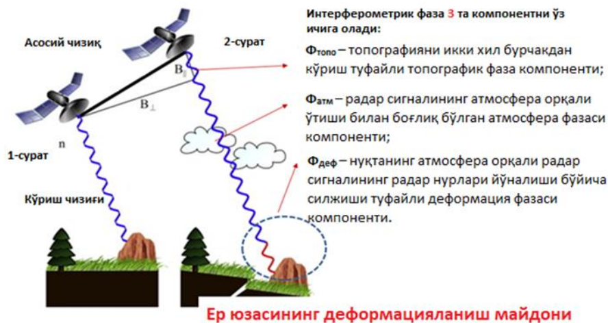
3-рasm. Interferometrik juftlik radar tasvirini olish sxemasi.
